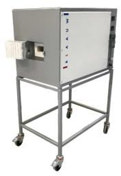
In a Blaauw gradient kiln, you can easily test your ceramic materials, clays, glazes, and clay bodies to different temperatures in a single firing. Set the maximum temperature and start the desired firing program with the friendly kiln user controller. During heating, a temperature gradient of 200-250°C (360-460°F) is established
